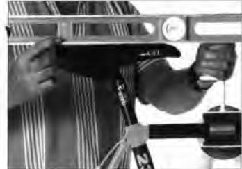
6 mm hex key. Starting with the saddle completely level (above), lower the nose slightly if you feel uncomfortable. Too far down will strain your arms and back. Too high up will hurt in time.
