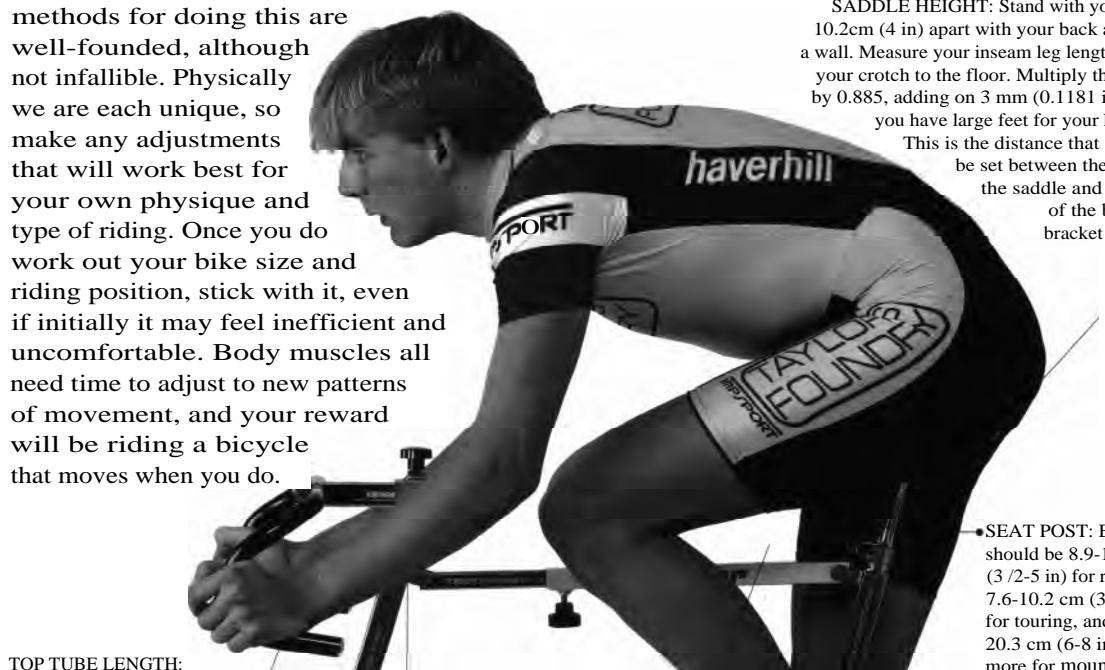
**TOP TUBE LENGTH:** The combined top tube and stem length should ideally position the handlebar so that in a normal riding position, the front hub axle is blocked from view by the handlebars.
