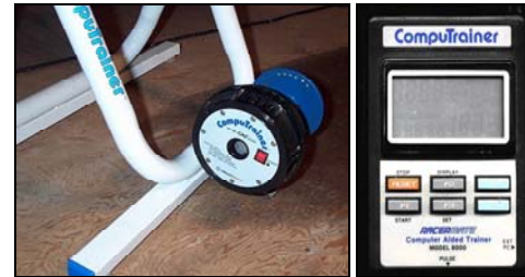
Figure 9. Stationary trainer power-measuring device. Manufactured by CompuTrainer.
