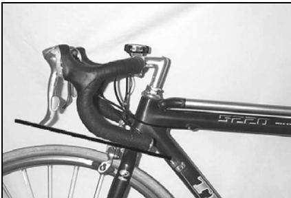
Figure 24. Handlebar and brake levers. Notice: Drops pointing to rear brake, brake lever tips inline with bottom of drops, and short stem.
